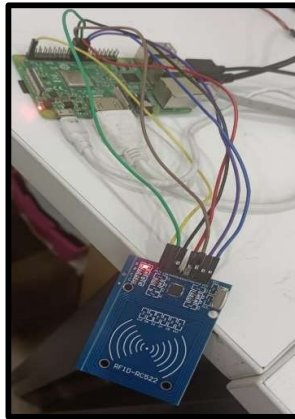
Fig. 19. Interfacing of Radio frequency Identification with Raspberry Pi Model 3 B
